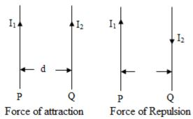
For finite (or) infinite length conductor,  $B = \frac{\mu_0 I}{2 \pi d}$ Force of attraction:  $F = \frac{\mu_0 I_1 I_2}{2 \pi d}$ Force of repulsion:  $F = \frac{\mu_0 I_1 I_2}{2 \pi d}$  The magnitude of force is same.
