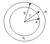
The potential difference between two coaxial cable is  $V = -\int_{b}^{a} E d r$
