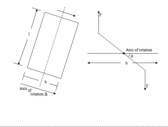
When a current loop is placed parallel to a magnetic field, force act on the loop that tend to rotate it. The tangential force multiplied by the radial distance at which it acts is called Torque or mechanical moments on the loop.
