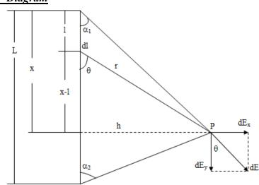
Electric Field for x component:  $E_x = \frac{\rho_l}{4 \pi \varepsilon} [\cos \alpha_1 + \cos \alpha_2]$ Electric Field for y component:  $E_y = \frac{\rho_l}{4 \pi \varepsilon} [\sin \alpha_1 - \sin \alpha_2]$ <u>Case 1</u>: If point is at bisector of the line, i.e  $\alpha_1 = \alpha_2 = \alpha$
