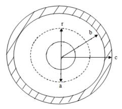
i) The field intensity within the solid inner conductor of radius ( $0 \le r \le a$ )
