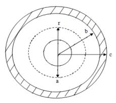
i) The field intensity within the solid inner conductor of radius  $(0 \le r \le a)$
