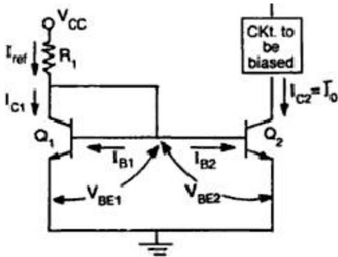
FIG:1 Current mirror circuit
