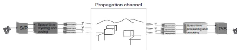
Figure 20.8 Principle behind spatial multiplexing.
