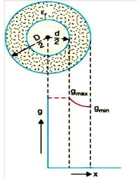
By definition, electric intensity is equal to potential gradient.
