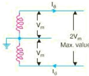
Max. voltage between conductors =  $2 V_m$
