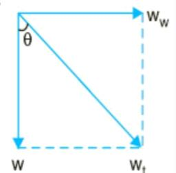
4. A transmission line has a span of 275 m between level supports. The conductor has an effective diameter of 1.96 cm and weighs 0.865 kg/m. Its ultimate strength is 8060 kg. If the conductor has ice coating of radial thickness 1.27 cm and is subjected to a wind pressure of 3.9 gm/cm<sup>2</sup> of projected area, calculate sag for a safety factor of 2. Weight of 1 c.c. of ice is 0.91 gm. (ND14, MJ16)
