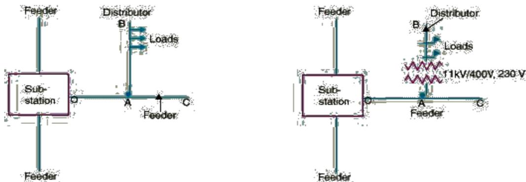
This is the simplest distribution circuit and has the lowest initial cost. However, it suffers from the following drawbacks :
