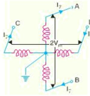
Max. voltage between outers  $A$  and  $B = 2V_m$
