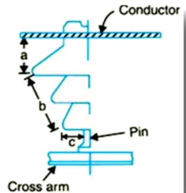
$$\text{Safety factor of insulator} = \frac{\text{Puncture strength}}{\text{Flash - over voltage}}$$
