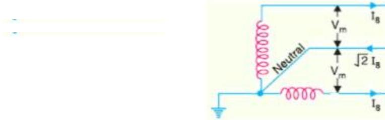
$$\text{Current in neutral* wire} = \sqrt{I_g^2 + I_g^2} = \sqrt{2} I_g$$
