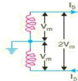
$$\text{Load current, } I_5 = \frac{P}{\sqrt{2} V_m \cos \phi}$$
