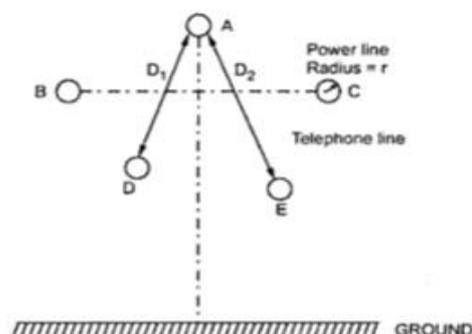
Consider the loop formed by the conductors A and D. Let the radius of each power line conductor be  $r$ . Let the distance between conductors A and D be  $D_1$  whereas the distance between conductors A and E be  $D_2$ . Assuming that in loop AD, A is contributing to the e.m.f. induced in D. If we neglect the internal flux linkages then the inductance of this loop is given by,
