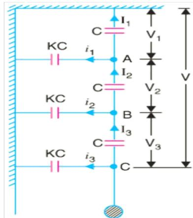
$$K = \frac{\text{Shunt Capacitance}}{\text{Self-capacitance}} = 0.11$$
