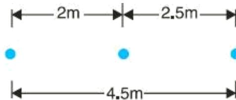
**Solution.** Fig shows the arrangement of conductors of the 3-phase line. The equivalent equilateral spacing is
