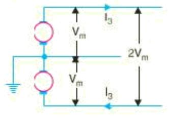
$$\text{Line losses, } W = 2I_3^2 R_3 = 2 \left( \frac{P}{2V_m} \right)^2 \times \rho \frac{l}{a_3} = \frac{P^2 \rho l}{2V_m^2 a_3}$$
