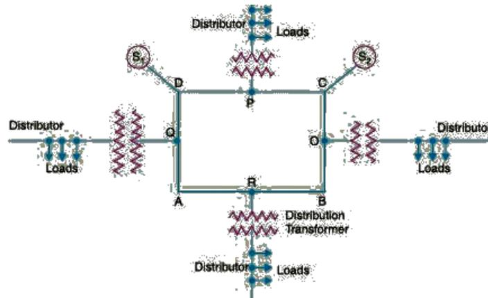
Distributors are connected to points *O*, *P*, *Q* and *R* of the feeder ring through distribution transformers.
