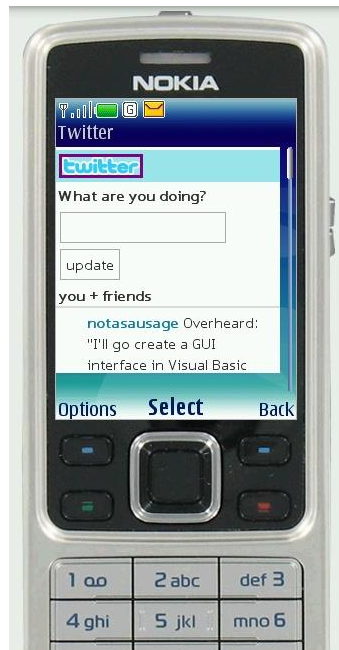
Figure 8-9. Example layout of a scroll-based application, where the user had to press the D-pad past each link to scroll the page
