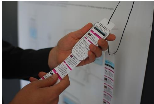
Figure 7-11. A paper prototype, where the interaction is nothing more than drawings on note cards
