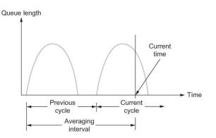
> Average queue length is measured over a time interval that includes the
