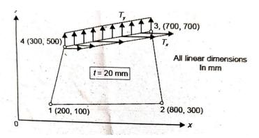
3. For the element shown in the fig, determine the Jacobian matrix (Nov Dec 18)
