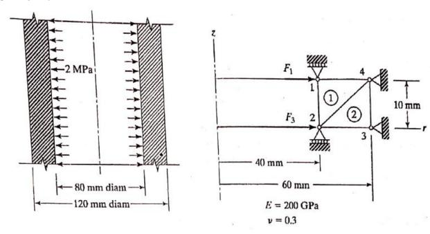
8. For a plane stress element shown in fig, the displacements  $(u_1, v_{1)}$ ,  $(u_2, v_{2)}$ ,  $(u_3, v_{3)}$  are (2, 1), (1,1.5) and (2.5, 0.5) respectively. Determine the element stress. Assume  $E = 200 \, \text{GN/m}^2$ ,  $\mu = 0.3$  and t = 10 mm, all co-ordinates are in mm. (Nov Dec 18)
