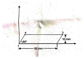
2. The quadrilateral element shown in fig is 20 mm thick and is subjected to surface forces  $T_x$  and  $T_Y$ . determine the expressions for its equivalent nodal forces if  $T_x$  and  $T_Y$  are  $10 \text{ N/mm}^2$  and  $15 \text{ N/mm}^2$  respectively (Apr May 19)
