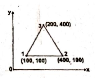
9. For the triangular element shown in the fig, assuming plane stress condition obtain strain-displacement matrix take poisson's ratio is 0.3, young's modulus is  $30 \times 10^6 \text{N/mm}^2$  and thickness is 0.1 mm. (Nov Dec 16)
