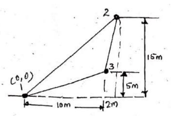
10. Compute strain displacement and stress, strain matrices for axisymmetric triangular element as shown in the fig, take poisson's ratio is 0.25, young's modulus is
