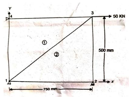
4. Calculate the element stresses for the axisymmetric element shown in fig, the nodal displacements are  $u_1$  = 0.02 mm,  $w_1$  = 0.03mm,  $u_2$  = 0.01,  $w_2$  = 0.06,  $u_3$  = 0.04 mm,  $w_3$  = 0.01 mm, take E = 210 GPa,  $\mu$  =0.25 (Nov Dec 18)
